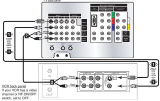
Figure 3. Connecting the VCR Audio/Video.
